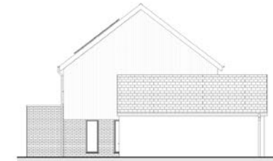
P6 Eastern elevation garage 1 : 100
